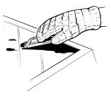
**Note:** Using a razor scraper will not damage the surface if the 30° angle is maintained.
