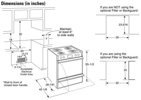
**Note:** Range may be placed with 0" clearance (flush) at the back wall and side walls if the range side trims extend beyond the cabinet fronts at least 1/4". (Self-clean models only.)
