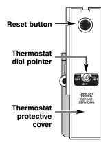
The illustration at the left shows the temperature adjustment dial used for setting the water temperature.
