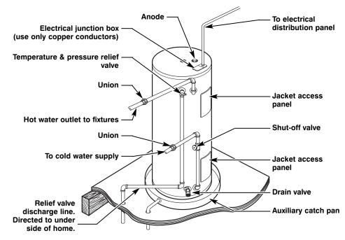
NOTICE: Do not apply heat to the HOT or COLD water connections. If sweat connections are used, sweat tubing to adapter before fitting adapter to the water connections on heater. Any heat applied to the water supply fittings will permanently damage the dip tube.
