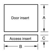
When using GPF325 1/4" custom dishwasher door and access panel kit. When using GPF375 3/4" custom dishwasher door and access panel kit.
