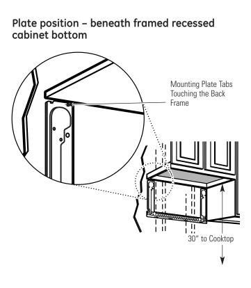
Your cabinets may have decorative trim that interferes with the microwave oven installation. Remove the decorative trim to install the microwave oven properly and to make it level.
