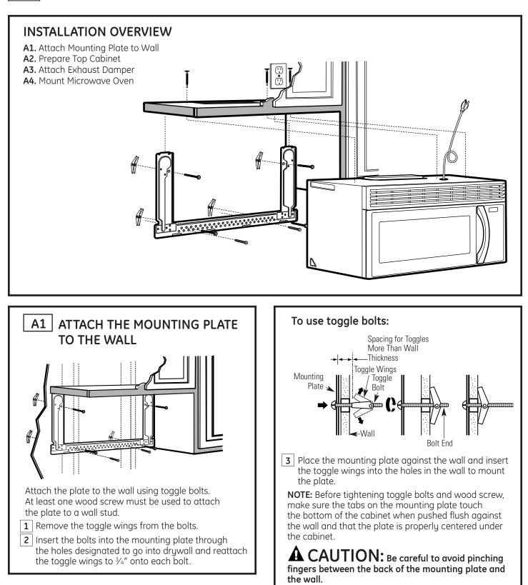
**4** Tighten all bolts. Pull the plate away from the wall to help tighten the bolts.
