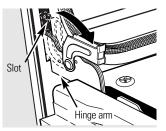
Hinge lock (unlocked position)
