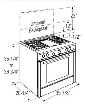
Clearances between range and side wall or combustible material must be at least 12" on each side.
