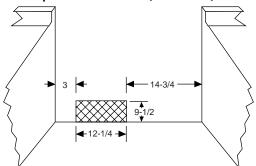
The electrical connection must be located in the shaded area shown.
