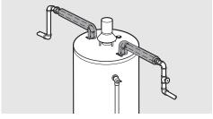
Typical horizontal piping arrangement
