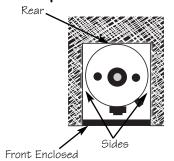
**A WARNING: Combustible** construction refers to adjacent walls and ceilings and should not be confused with combustible or flammable products and materials. Combustible and/or flammable products and materials should never be stored in the vicinity of this or any gas appliance.
