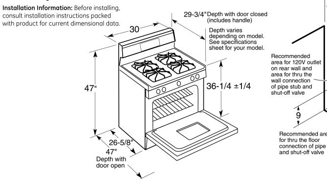
Recommended common area for gas outlet and electrical outlet 30 2-1/2 Recommended area connection of pipe stub
