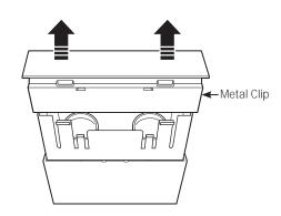
**WARNING** — The metal clip must be replaced or the heat from the bulb could damage the refrigerator.
