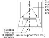
Side-by-Side Installations Install two ovens in separate cutouts. Door handles should face toward each other Center Line 30.5" (77.5 cm) Cutout -Cutout observe all observe all dimensions and dimensions and requirements - 2" (5.1 cm) Min
