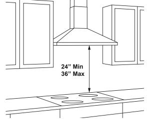
The vent hood must be installed 24" min. above the cooking surface. For optimal performance, installing the hood more than 36" above the cooking surface is not recommended. The hood installation height above the cooking surface depends upon the ceiling height. The telescopic duct cover conceals the ductwork running from the top of the hood to the ceiling.
