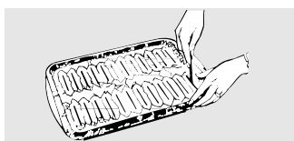
Cut slits in the foil just like the grid.
