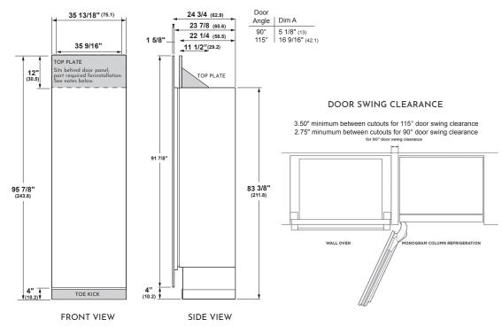
Designer Collection Top Plates & 4" Toe Kicks are available in different widths to avoid seams when combining columns. Top Plates must be installed onto the appliance before installing into cabinetry. See Top Plate Installation Guide. Due to 96" finished height, this part is required for proper installation.
