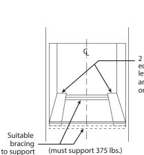
2 x 4 or equivalent runners level with bottom of cutout and flush with sides of cutout or solid bottom floor.
