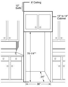
"The rough-in dimension of 70-1/4" is minimum and is measured from the finished floor to top of opening (or the underside of the overhead cabinets). For Models with Trim Kit. If trameless style cabinets are planned for above the refrigerator, you may need to consider adding a maximum of 1/4" (70-1/2") to height of opening to allow additional clearance between cabinet doors and top of refrigerator trim when cabinet doors are in one notified.
