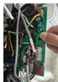
6. Pull out the PCB and unplug the refrigerant leak sensor from CN3.
