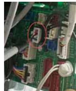
4. Pull out the PCB and unplug the refrigerant leak sensor from CN3.
