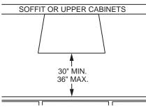
In this installation, the ductwork running from the top of the hood will be concealed in the soffit or upper cabinetry. **NOTE:** Clearances may vary due to type of cooking product and local codes. Check with local inspectors to be sure standard is applicable.
