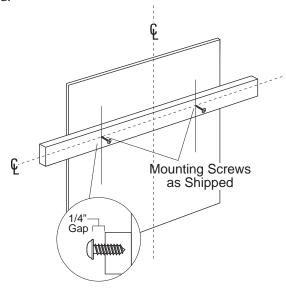
■ Adjust depth of supplied mounting screws in the wood support until they protrude 1/4" forward. This 1/4" gap will provide clearance to hang the hood.
