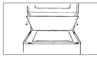
Remove two Phillips-head screws at top of panel.
