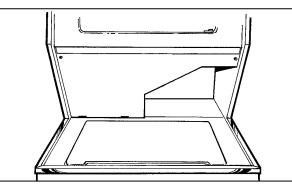
Lift access panel up until tabs at sides of panel slip out of slots at sides of dryer.
