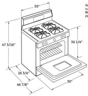
Recommended area for 120V outlet on rear wall and area for through-the-wall connection of pipe stub and shut-off valve.
