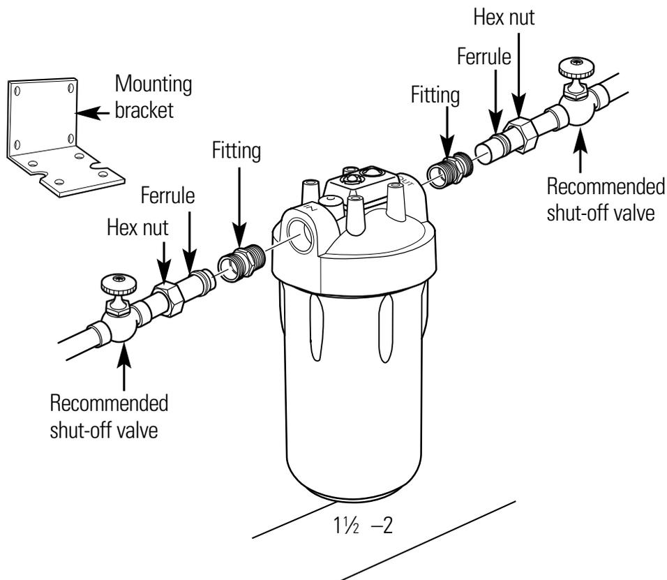
**Note:** Can be installed undercounter (as shown), in basement, or other convenient location. Before installing, see installation instructions packed with product for complete details.
