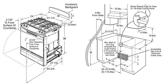
You must use the rear filler strip kit shipped with the range or the optional accessory backguard (JXS31, JXS32, JXS33, JXS34) when installing these ranges.
