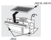
For installation between cabinets only; not for end-of-cabinet installation. Each kit contains two 3"-wide filler panels.
