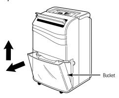
**Use a hose.** Water can be automatically emptied into a drain by attaching a length of thin-wall rubber or plastic tubing with an inside diameter of 1/2 inch. Use a screwdriver to remove the knockout at the back. Attach the tubing to the connector through the hole.
