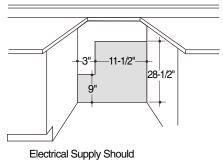
Electrical Supply Should Enter From Back Wall In Shaded Area.
