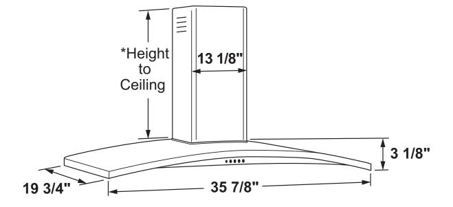
\*The supplied duct cover fits 7' 11" to 10' 2" ceiling heights (10' 6" in recirculation mode)
