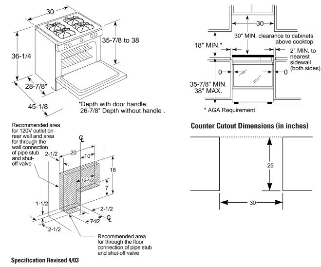
Note: Model JGSP23BEY is shipped with special "vented" rear filler strip. Post form countertops may not be used when installing this range. The filler strip (provided) or optional backguard kit is required for installation.
