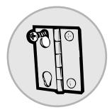
Loosen top screw from each hinge on the dryer face half way. With one hand holding the top of the door and the other hand holding the bottom, remove the door from the dryer by lifting it **UP** and **OUT**.
