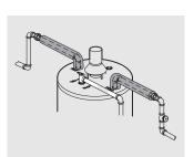
Typical horizontal piping arrangement
