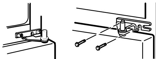
3.3 Remove the tape and tilt the door away from the cabinet. Lift the door from the pin in the bottom hinge bracket. (If the plastic washer sticks to the door bottom, put it back on the hinge.)
