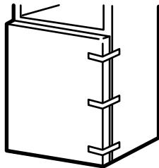
3.2 Using a 5/16" hex-head socket screwdriver and a 5/16" open-end wrench, remove the two screws holding the center hinge (and the shim glued to it) to the cabinet. Lift the center hinge to free its pin from the socket in the top of the door, and set hinge and screws aside. **Be careful not to lose the center hinge spacer and washer.**
