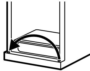
3.7 Take one of the screws removed in step 2 and start it in the outermost screw hole on the opposite side. Do not drive it all the way down—leave enough space under the screw head for thickness of shim and bracket.
