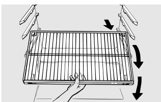
**To remove a full-width shelf when the fresh food compartment door cannot be opened fully,** lift the rear of the shelf, pull forward and down, tilt the shelf and take it out.
