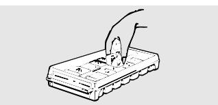
**For only one or two ice cubes,** leave the tray right-side up, twist both ends slightly and remove desired number of cubes. **Wash ice trays and storage bin in lukewarm water only.** Do not put them in an automatic dishwasher.
