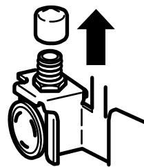
9.3 Place the compression nut and ferrule (sleeve) onto the end of the tubing as shown.
