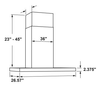
The vent hood must be installed 24" min. above the cooking surface. For optimal performance, installing the hood more than 38" above the cooking surface is not recommended. The hood installation height above the cooking surface depends upon the ceiling height. The telescopic duct cover conceals the ductwork running from the top of the hood to the ceiling.
