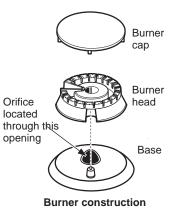
B. Using a 7 mm or 9/32" nut driver, remove the top burner orifices. These may be accessed through the burner opening in the base.
