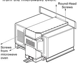
Place the top bracket on top of the upper duct, with the opening on the top bracket lined up with the opening on the duct.
