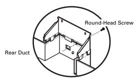
Remove all loose items, including the turntable and turntable support, from the microwave oven. Carefully turn the oven upside down. Remove three screws (one from control side, and two from bottom rear) from microwave oven cabinet. Place the bottom duct assembly on the microwave oven bottom and fasten with four round-head screws and the screws just removed from the microwave oven. Turn the microwave oven right side up, being careful not to bend the bottom duct flange.
