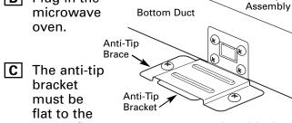
cutout floor to engage correctly with the anti-tip brace as shown. Carefully slide the microwave oven back, engaging the anti-tip brace. Make sure the power cord is not mashed or cut as you slide the microwave into place.
