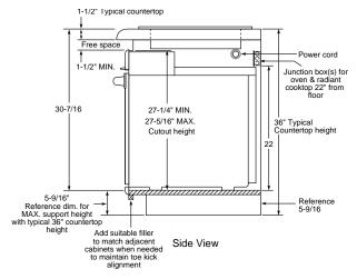
This installation is to achieve minimum gap between bottom of countertop and control panel.
