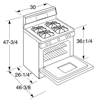
\*Dimension From the wall to the front of the closed door handle is 29".
