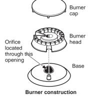
B. Using a 7 mm or 9/32" nut driver, remove the top burner orifices. These may be accessed through the burner opening in the base.
