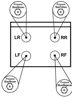
To prevent leakage, make sure the orifice spuds are securely screwed into the gas supply tubes.
