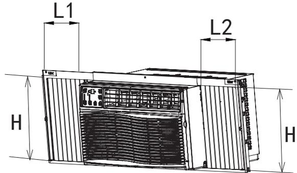
B. Cut the foam insulation to the measured length of the left and right side accordion. **NOTE:** Be sure to measure each accordion because the length could be different on each side.
