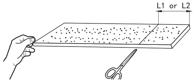
C. Remove adhesive from back of foam insulation. Stick the foam insulation onto the left and right accordion, and inside of the frames.
