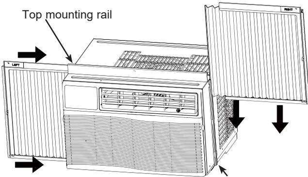
E. Slide the left and right accordion panels into the top and bottom mounting rails.
