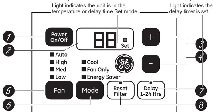
NOTE: The display always shows the room temperature except when setting the Set temperature or the Delay timer.
