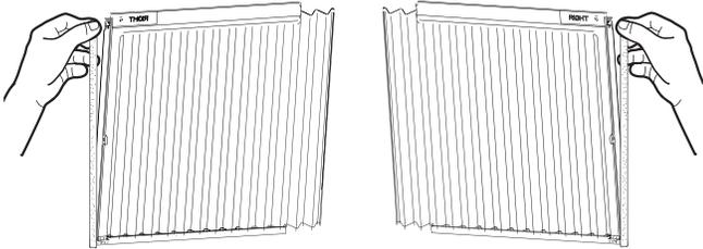
D. Slide the free end of the accordion panel into the side panel rails. Slide the panel down. Be sure to leave enough space to slip the top and bottom of the frame into the rails on the cabinet.
