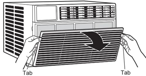
**CAUTION** DO NOT operate the air conditioner without a filter because dirt and lint will clog it and reduce performance.
