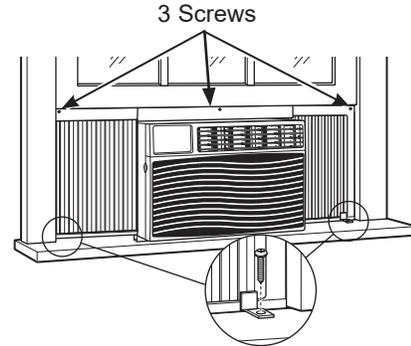
B. Extend the left and right accordion panels to the vertical window sashes and attach 3 screws through the holes in the upper panels, as appropriate.
