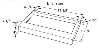
A stainless steel liner is shipped with each hood insert. This non-combustible liner protects the underside of the canopy.
