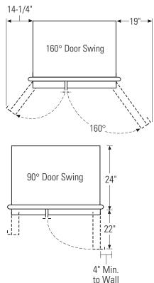
Allow 19" minimum clearance on the fresh food side for a full 160° door swing and pan removal. Allow 14-1/4" clearance on the freezer side for removal of ice bin.
