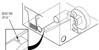
Through the rear opening, locate the tab in the middle of the appliance base. Lift the tab to about 45° using a flat blade screwdriver.
