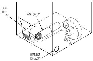
Reconnect the cut portion (A) of the duct to the blower housing. Make sure that the fixing hole is aligned with the tab in the base. Use the screw saved previously to secure the duct in place through the tab on the appliance base.
