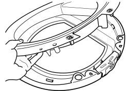
18. Place the outer door onto the inner door.
