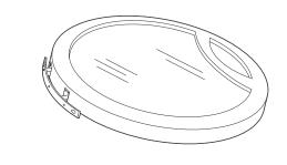
20. Turn the door over and fasten the outer door to the inner door using the 6 large tapping screws (#10).
