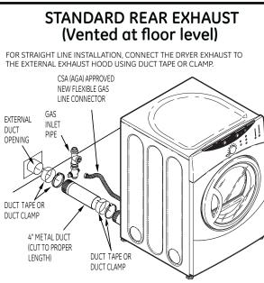
NOTE: WE STRONGLY RECOMMEND SOLID METAL EXHAUST DUCTING. HOWEVER, IF FLEXIBLE DUCTING IS USED IT MUST BE UL-LISTED METAL NOT PLASTIC.
