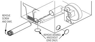
Detach and remove the bottom or left side knockout as desired. Remove the screw inside the dryer exhaust duct and save. Pull the duct out of the dryer. Protect sharp edges around the knockout and exhaust opening with the tape.
