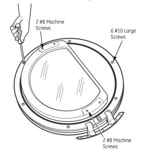
6. With the screws removed, turn the door over and separate the silver cover part of the door from the door frame and set aside.
