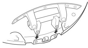
12. Loosely fasten the hinge assembly to the edge using 2 machine screws (#8).
