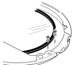
10. Remove the hinge assembly by removing the 2 machine screws (#8) that fasten it to the frame. Pull the hinge assembly out and set it aside.
