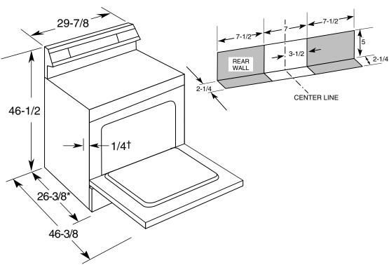
\*Dimensions from wall to front of closed oven door handle. Dimensions from wall to front of closed oven door handle is 28".
