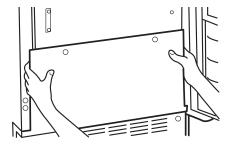
**4.** Remove dirt and lint from the condenser fins and the unit compartment with a brush attachment attached to a vacuum cleaner.
