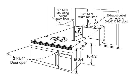
**Note:** Requires 120V grounded outlet. Electrical receptacle must be located in cabinet above Spacemaker microwave oven. No additional wiring, venting or cabinet rebuilding necessary in many cases. Complete detailed, easy-to-follow installation instructions and convenient full-size templates are packed with the Spacemaker microwave oven.
