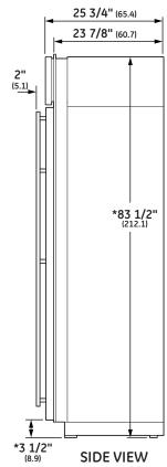
\* Shipping height. Use leveling legs and wheels for maximum 1" height adjustment from shipping height.
