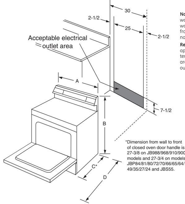
**Note:** Conforms to U.L. requirements for 0" spacing for adjacent walls below countertops. To reduce possibility of scorching of walls, it is recommended a minimum of 1-1/2" spacing be allowed from adjacent side walls to allow for possible extended, high-heat, no-load heating element operation.
