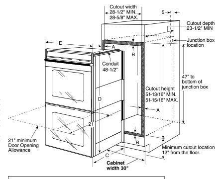
MOST 30" WALL CABINETS CAN BE USED WITH THIS UNIT. THE OPENING BETWEEN THE INSIDE WALLS MUST BE AT LEAST 28-1/2" WIDE.
