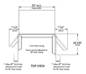
\*\* These refrigerators are equipped with a 2-position door stop. The factory-set 115° door swing can be adjusted to 90° if clearances to adjacent cabinets or walls is restricted. Allow a 15" minimum clearance to wall for pan removal. If the 90° door stop position is used, pan access is maintained, but pan removal is restricted.
