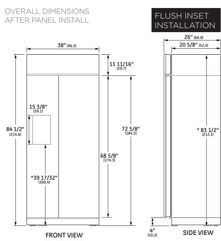
Use leveling legs and wheels for maximum 1" height adjustment from shipping height. Nominal installation height is 84".
