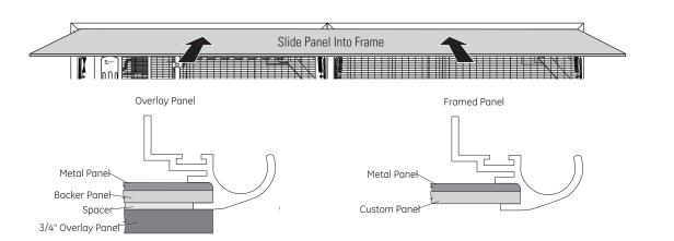
• Slide framed or overlay panel over the metal backer panel and into the trim. If necessary, tap with a wood block until panel slips under the top trim piece.
