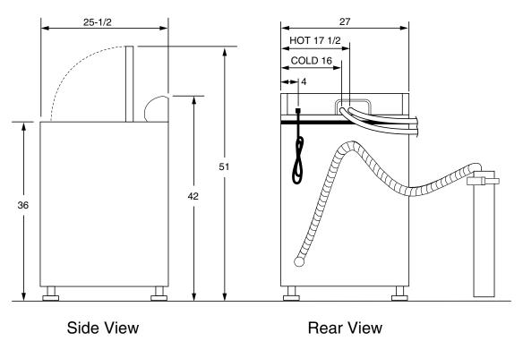
**Circuit Requirements:** An individual, properly-grounded branch circuit, with a three-prong grounding-type receptacle, protected by a 15 or 20 amp circuit breaker or a time-delay fuse, is required.
